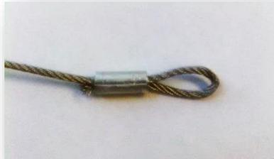
Cable pull rope end is looped through the T-model activator cotter pin manual release and crimped with a choice of stainless or tin-plated copper oval sleeve. Cable bulkhead fittings must be properly anchored. Thermal switch is an optional electrical contact to indicate released status.
