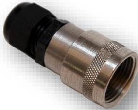
The cable adapter can be used for connecting releasing circuit wiring from a junction box to the 3/4" threaded coupling on electric operation Stat-X aerosol generators. It has a cable gland that will tighten around releasing circuit wiring.
